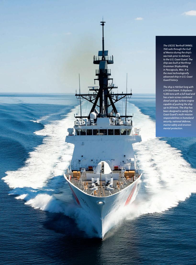
has a twin-screw combined diesel and gas turbine engine capable of pushing the ship up to 28 knots. The ship has been designed to satisfy the Coast Guard's multi-mission responsibilities in homeland security, national defense, marine safety and environ-
